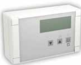
CT – Total Control Suitable for all models from Optima to Max (except Minibel and Eco). Auxiliary devices: anti-freeze sensor, door contact, thermostat, etc... Time programmer: 3 ON/OFF for each different day of the week. Digital display with hour, fan speed, heating stage, temperature... Multilanguage display 9 languages. Manual or automatic functioning with programmable behaviours.
