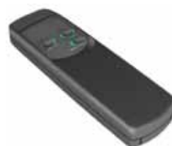
CT – Total Control Suitable for all models from Optima to Max (except Minibel and Eco). Auxiliary devices: anti-freeze sensor, door contact, thermostat, etc... Time programmer: 3 ON/OFF for each different day of the week. Digital display with hour, fan speed, heating stage, temperature... Multilanguage display 9 languages. Manual or automatic functioning with programmable behaviours.
